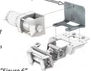
“Figure 6” Exploded View of a 2-Hole Mounted Winch
