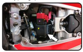
Locate and disconnect fender sub-harness connector.
