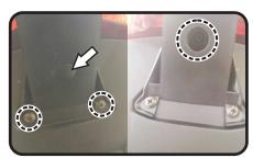
4. Disassemble the stock fender assembly and remove the left and right turn signals.
