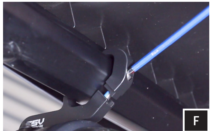
F. Using a T5 hex key tighten clamp until it secures to cage.
