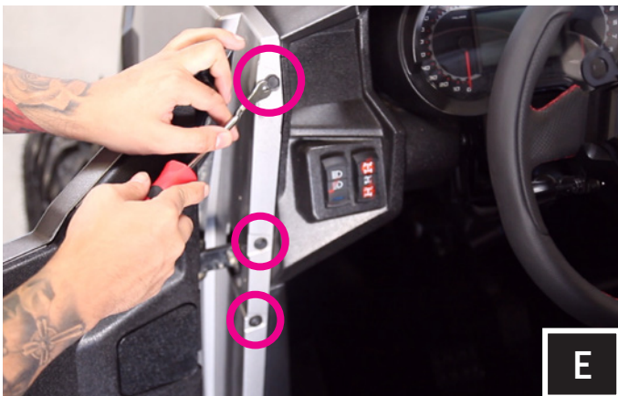
E. Remove top push pins as well as the lower T30 Screw (this will allow for easy removal of top dash panel).
