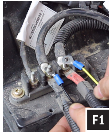
F. At the Bus Bar terminal located under the hood, unscrew the nut on the second position terminal and attach the black Ground wire. Refasten the nut. Then connect the yellow Power wire to either the constant terminal (F1) or the accessory terminal (F2). Refasten the nut.
