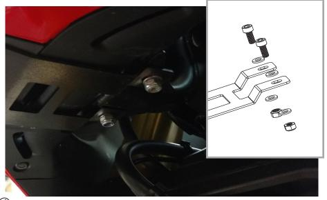
Use (2 qty) M6 x 14mm socket cap screws, (4 qty) M6 washers, and (2 qty) M6 lock nuts to loosely attach bracket to the mounting points under the nose of the bike, as shown.
