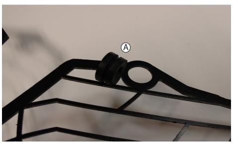
1 Install four (4) rubber grommets into headlight guard. (A) Use care to not rip the rubber. **!TIP** a dab of water will help them slide into place, a small dull flathead screwdriver is a good tool to use.
