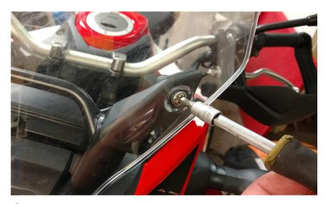
Use 5mm allen tool and remove four(4) windscreen screws. Remove windscreen. Save these for reinstallation.
