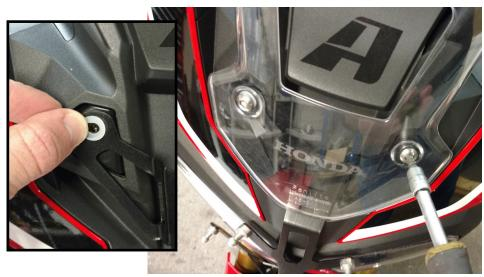
(5) Attach bracket at upper mount points with windscreen. Use one M6 nylon washers on top of bracket at each screw as shown. Screw loosely in place.
