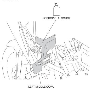
4. Peel off the adhesive backing on the left wind deflector as shown.
