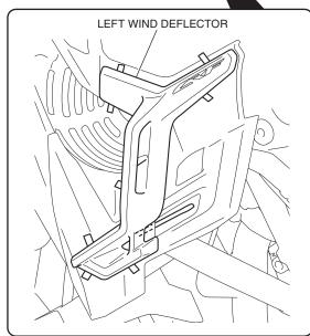
6. Remove the adhesive backing as shown.
