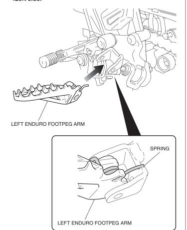
7. Install the pivot pin and split pin as shown.
