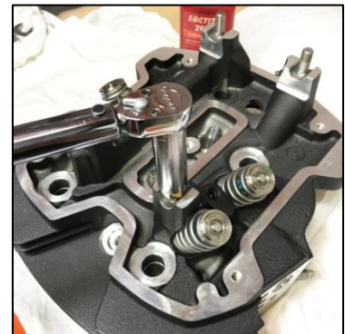
Torque stud to 3-5 Ft. Lbs
