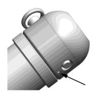
3) Install the plastic top using the removable pin. **Important:** One side of the puck has a small hole drilled beneath the main hole. Install the pin so that the end of the pin with the ball is
