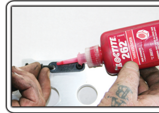
Apply Loctite to block off plate bolts
