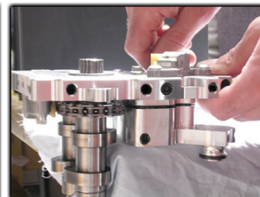
Bolt oil pump to camplate finger tight DO NOT use loctite or hardening compound
