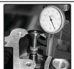
Installed valve spring height is critical!
