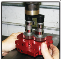
Line up timing marks, press in camshafts using lube and the proper tools
