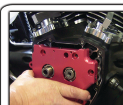
Wiggling assembly while rotating engine back & forth will aid alignment & installation
