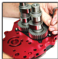
Install bearing retainer plate using loctite
