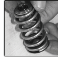
Clean & inspect new springs & hardware
