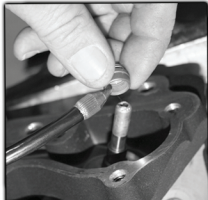
Install valve seals. Use protective sleeve on valve to protect seal during installation. Pre-lube seals with engine oil prior to installation
