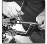
Remove original valve springs & hardware
