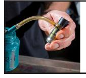
Pump up each lifter prior to installation.
