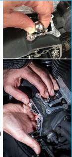
NOTE: Recommended lifter to lifter bore clearance 0.001"-0.0015". The closer the clearance is to 0.001", the higher the oil psi at the lifter will be, producing a quieter, happier valvetrain.
