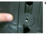
Install your new Flare<sup>™</sup> Windshield with the hardware removed in step 7 and torque fasteners to factory specifications.
