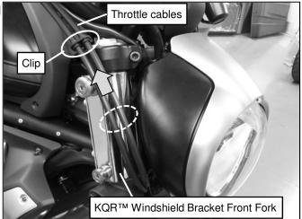
5. Remove the clip from the throttle cables and re-install it at a higher position just above the front fork tube as shown.
