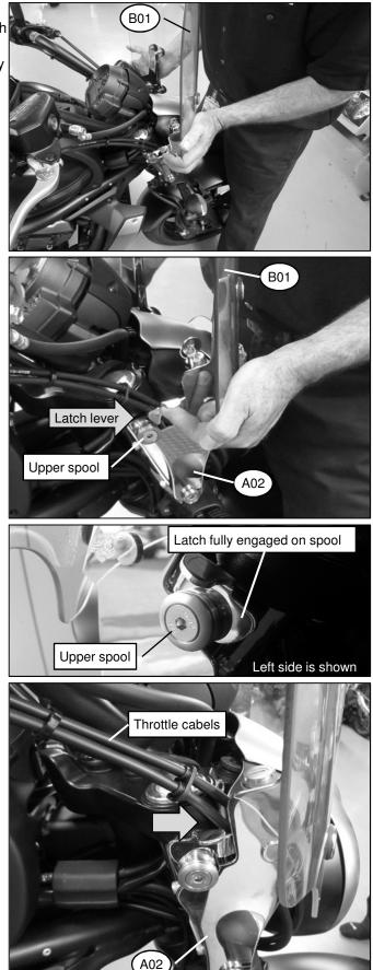
8. To remove windshield, lift up on the spring-loaded Left Latch Lever and Right Latch Lever simultaneously until they clear the upper spools, then pull firmly forward until the latches fully clear the spools and lift the windshield clear of the lower spools.
