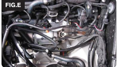
10 Attach the connectors from the PCFC to the stock wiring harness and injectors as shown in Figure E.
