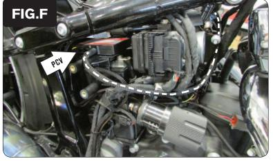
11 Secure the PCV module to the top of the battery on the right side using the supplied Velcro (Fig. F).
