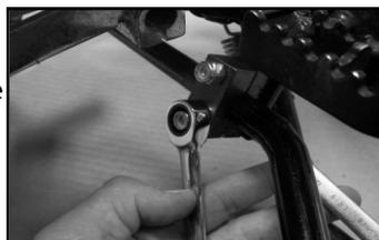
10.4 Make sure the spacing between the two mounting blocks stay the same. You can do this by counting the amount of turns made when tightening the nuts. **Stop tightening** when the axle is snug but can be moved up or down with a little pressure.
