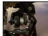
3.1 Make sure you install the Axle Mounting Plates behind (bottom side) of the foot pegs. (If your motorcycle has an off-set foot peg mount, you may need to place one Axle Mounting Plate behind one foot peg and the other in front of the other peg.)
