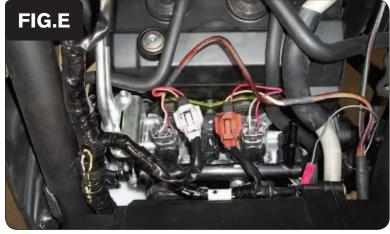
7 Plug the PCV in-line of the stock injectors and wiring harness (Fig. E)
