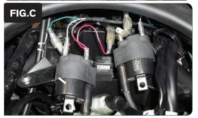
5 Plug the PCV in-line of the ignition coils and wiring harness (Fig. C).
