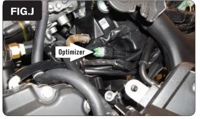
11 Unplug the stock O2 sensor and plug the supplied O2 Optimizer into the wiring harness (Fig. J).
