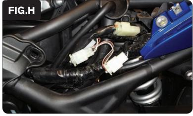
10 Plug the PCV in-line of the stock CPS and wiring harness (Fig. H).
