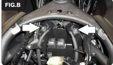
3 Remove the bolts that hold the ignition coils in place (Fig. B).
