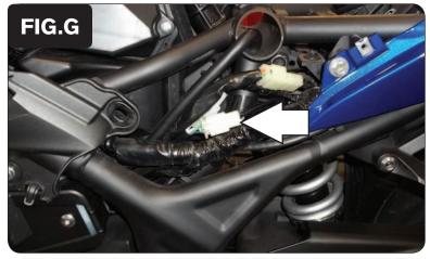
9 Unplug the crank position sensor connector (Fig. G).
