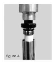
7. Once the fork tube is completely un-threaded from the cap (Figure 3) carefully release the press, allowing the fork spring to safely extend fully (Figure 4)
