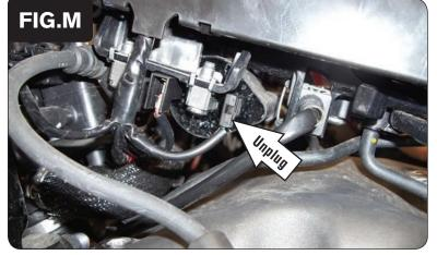
17 From the left side of the frame, unplug the GREEN/RED (signal) wire from the right cylinder ignition coil (Fig. M).
