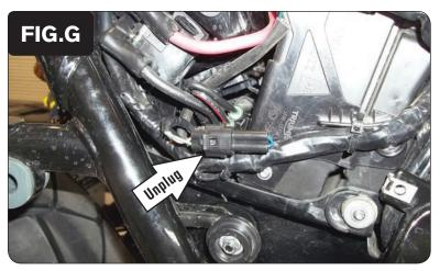
11 Unplug the crank position sensor connectors on the right side of the bike (Fig. G).
