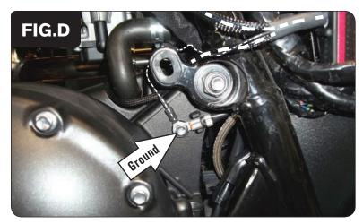
8 Use the stock common ground bolt on the left side of the engine case to secure the PCV ground wire with the small ring terminal (Fig. D).
