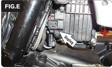
9 Unplug the throttle body servo connector on the right side of the bike (Fig. E).
