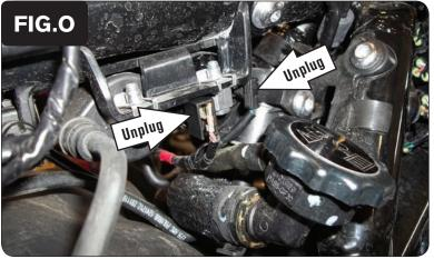
19. From the right side of the bike, unplug the BROWN (power) wire and the GREEN/BLUE (signal) wire from the left cylinder ignition coil (Fig. O).
