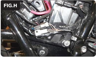
12 Plug the PCV wiring harness in-line of the stock crank position sensor connectors (Fig. H).
