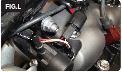
16 Plug the pair of PCV connectors with YELLOW colored wires in-line of the right fuel injector and the stock connector (Fig. L).
