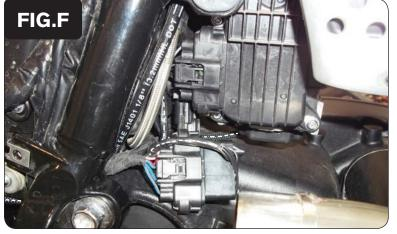
Plug the PCV wiring harness in-line of the throttle body servo and stock wiring harness (Fig. F).
