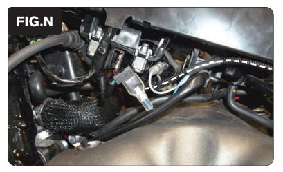
Plug the pair of PCV wires with spade connectors (BLUE and WHITE/BLUE wires) in-line of the right cylinder ignition coil and the stock GREEN/RED wire (Fig. N).
