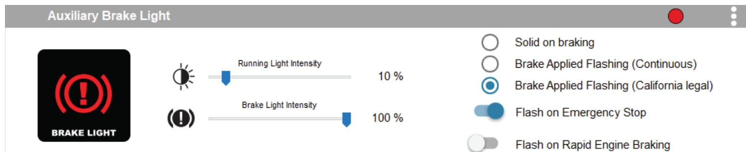
The Auxiliary Brake Light settings interface includes a 'BRAKE LIGHT' icon and two intensity sliders: 'Running Light Intensity' at 10% and 'Brake Light Intensity' at 100%. On the right, there are five toggle options: 'Solid on braking' (off), 'Brake Applied Flashing (Continuous)' (off), 'Brake Applied Flashing (California legal)' (on), 'Flash on Emergency Stop' (on), and 'Flash on Rapid Engine Braking' (off).
