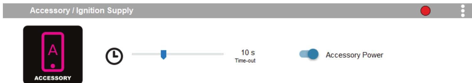
The Accessory / Ignition Supply settings interface includes an 'ACCESSORY' icon, a clock icon, a slider set to '10 s Time-out', and a toggle switch for 'Accessory Power' which is turned on.
