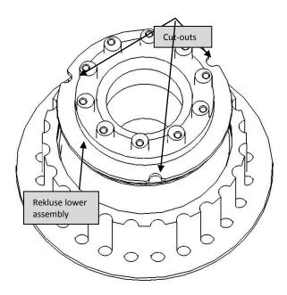
**20.** Using a pair of mechanics gloves (the edges of the ring can be sharp and may cut you), install the retaining ring into the Rekluse Center Clutch ring groove.
