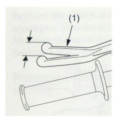
**Tip:** Use one finger with light pull when checking for lever free play. This will make it easier to distinguish between the light resistance of the lever return spring and the significant resistance felt when disengaging the Rekluse pressure plate.
