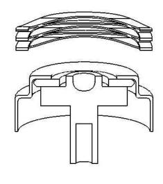
**26.** Install the C200 wave spring (if used by chosen configuration) on top of rotating hub into the locating pocket.
