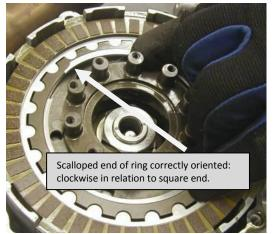
Threading retaining ring into groove
