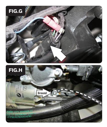
11 Using the supplied Posi-Tap connect the BLUE wire of the PCV to the PURPLE/BLACK wire of the gear position sensor connector (Fig. G).
