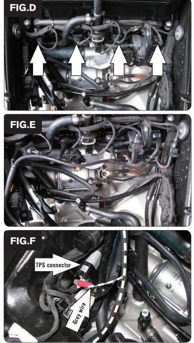
7 Unplug the stock wiring harness from each lower primary fuel injector (Fig. D).
