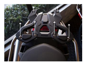
Remove OEM luggage rack. Use T30 driver to remove 6 button head cap screws.
