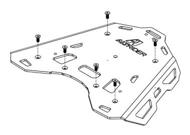
Align AltRider Luggage rack over OEM bolt hole locations, install (6) M6 flat head fasteners in locations shown.
