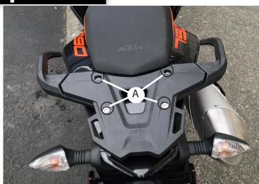
① Option#2, Install AltRider Rack without OEM rack or handles. First, remove (4) OEM fasteners (A) from rack using T40 driver . Remove rack, and handle peices.
