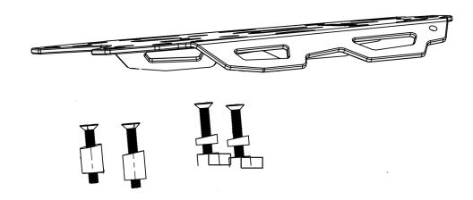
Place the AltRider provided spacer combo as shown with 8mm angled spacers stacked on top of 7.96 mm spacers in the rear location, and 25mm angled spacers. Low point of the spacer should face forward (towards the seat).
