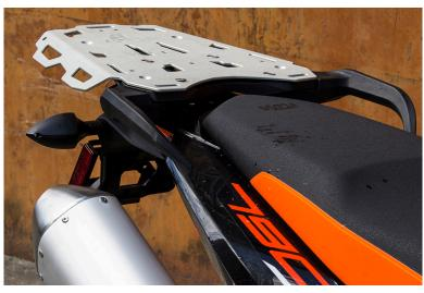
Place the AltRider rear rack on top of the OEM Rack and handles, replacing the two forward OEM fasteners with M8x60 and M8x55 fasteners.
