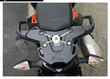
Option #1, install AltRider rack directly on top of OEM rack.
