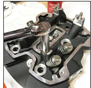
Torque stud to 3-5 Ft. Lbs
