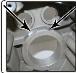
Verify Intake lobes of camshafts clear engine case Crank bearing boss & lifter bosses
