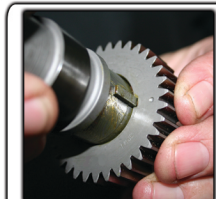
Line up gear with camshaft
