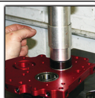
Press in new cam bearings using the proper tools use high pressure press lube on bearings & bores
