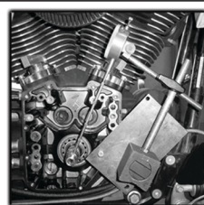
Dial indicator with Magnetic base
