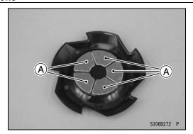
• Stick the crankcase ring [1] to the clutch cover [A].
