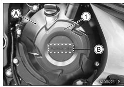
• Stick the crankcase ring [2] to the alternator cover [A].
