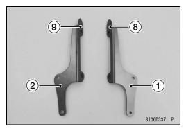
• Install the brackets [1] [2], and temporary tighten the bolts [7].
