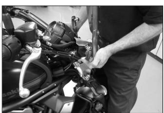
9. If desired, use the key to lock the Right Latch on the Right Windshield Bracket (A02).
