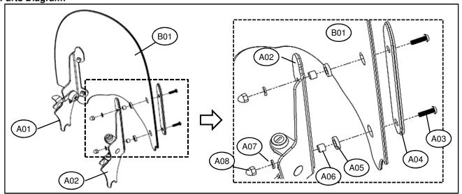
Note: Fitment of KQR™ Windshield Bracket requires prior installation of KQR™ Windshield Bracket Front Fork
