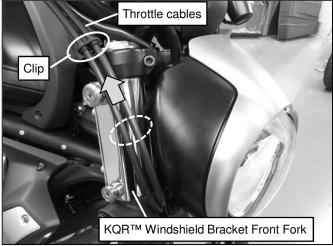
6. Hold the Windshield assembly in both hands with front side toward you and position the lower fork of each Windshield Bracket onto the lower spools of the Windshield Bracket Front Fork (99994-0546) previously installed, then move the upper part of the windshield back until the upper latches contact the upper spools.
