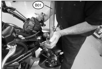
7. Lift up on the spring-loaded Left Latch Lever and Right Latch Lever simultaneously until they clear the upper spools, then press firmly rearward until the latches fully engage the spools on both sides.
