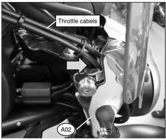
8. To remove windshield, lift up on the spring-loaded Left Latch Lever and Right Latch Lever simultaneously until they clear the upper spools, then pull firmly forward until the latches fully clear the spools and lift the windshield clear of the lower spools.
