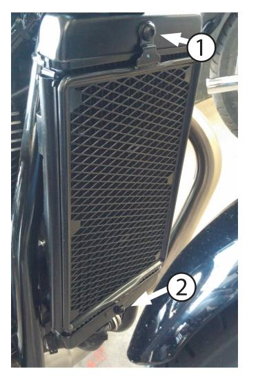
Use a 5mm allen tool to Remove the (2) button head fasteners from the OEM radiator guard. Remove the guard. Save the two fasteners for reinstallation.
