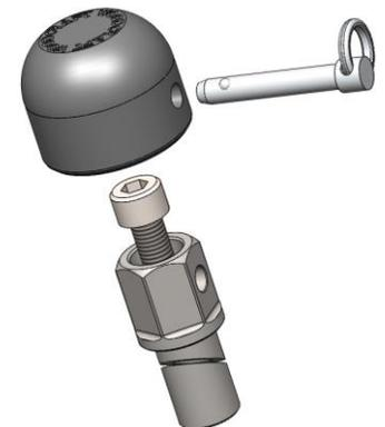
6) Install the plastic top using the removable pin. Be sure to orient the pin as done in step 3. To remove the axle, simply take the puck off the nut side. The nut will slide over the base and the main axle slider bases can remain installed.
