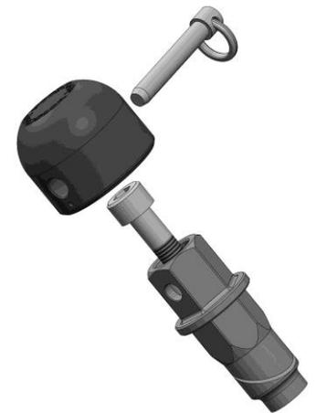
4) **Nut Side:** The nut side assembly can be installed with the axle nut in place. Thread the 8x25mm socket head bolt into the assembly until it is almost tight, leaving a small gap between the halves. Slide the assembly into the end of the axle and be sure that it is fully seated against the axle.
