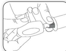
6. Draw the wire through the handlebar (it can be helpful to use a thin wire loop to pull it through), as far as possible. The wires should not be loose inside the handlebar when the BL 1000 PL is installed. Turn the BL 1000 PL counter-clockwise a few times and then insert it into the handlebar.
