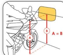
9. The proper alignment is necessary for safety when driving in traffic and a required component for vehicle approval; a vehicle with incorrectly aligned lights is easily not noticed.
