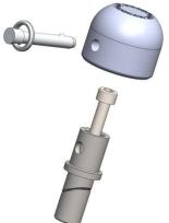
A note for racers: If your tech inspector wants you to safety wire these (most will not) then you simply need to orient the pins so that the pull on the pin is both clockwise and down (so that it acts to both tighten the bolt and pull the pin into the puck)
