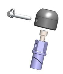
2) Tighten the 8mm allen bolt to lock the assembly in place. You should hold the he with a wrench while doing this to ensure you can fully lock the axle side in place.
