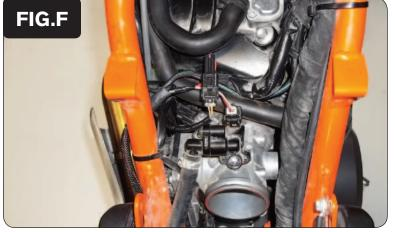
12 Plug the PCV in-line of the stock injector and wiring harness (Fig. F).
