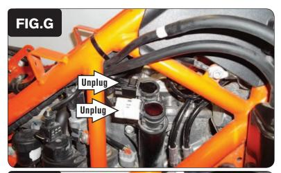
On the right side of the engine, locate and unplug the stock BLACK 2-pin connector from the inner coil stick and the stock WHITE 2-pin connector from the outer coil stick (Fig. G).
