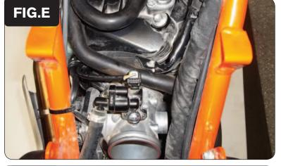
11 Locate and unplug the bike's Fuel Injector (Fig. E).
