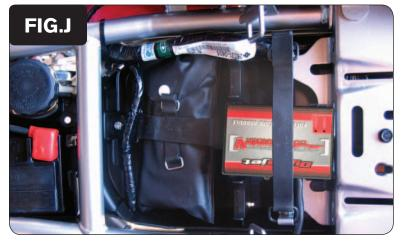
16 Secure the PCV in the tail section using the stock rubber band (Fig. J).
