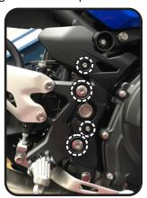
4. It is required to remove the swingarm bolt to replace left and right swingarm bracket plates. Place motorcycle in front wheel chock to center upright. Place floor jack under oil pan to lightly support engine and to unload rear suspension to ease removal of the swingarm bolt.
