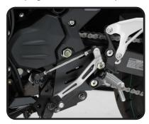
11. Apply thread lock to the stock footpeg bolts. Install right footpeg bracket to Yoshimura right rearset bracket. Torque to factory specification. Re-install right side swingarm bracket plate cover using the stock bolts. Secure right side fairing to fairing bracket using the stock bolt. Torque to factory specification.
