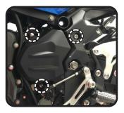
2. Remove the stock shift rod by loosening the shift rod locknuts. Remove the two bolts securing left footpeg assembly to left swingarm bracket plate.
