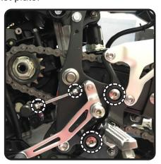
3. Remove the two right side swingarm bracket plate cover screws and remove cover. Remove the two bolts securing right footpeg assembly to right swingarm bracket plate.
