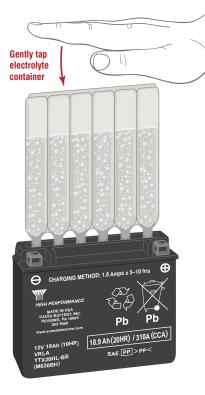
5. Remove the empty electrolyte container from the battery. Fully insert the strip of sealing caps (previously removed from the electrolyte container) into the battery filling ports. Make sure the strip of caps is fully inserted and flush with the top of the battery. Insert the caps by hand, do not use
