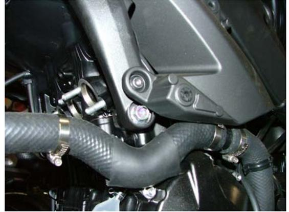
2) Attach the inner slider base to the motorcycle using the 10mm bolts provided, threading them in place of your motor mount bolt. Torque to OEM recommended specifications (consult service manual). The **left** side slider uses a spacer between the base and the frame.
