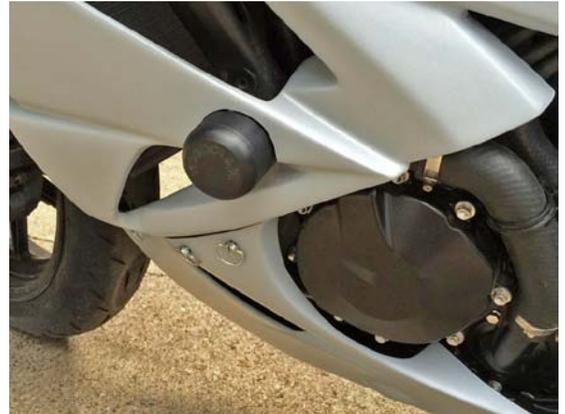
5) Slide the plastic slider over the top of the base and secure in place using the 8mm countersunk bolt provided. The bolt passes first through the non threaded hole and then screws into the threaded hole on the far side of the base. The plastic is undersized on the far side of the slider to act as a locknut for the bolt.
