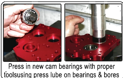
Verify bearings are flush with camplate
