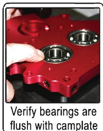
Press in camshafts use lube & proper tools
