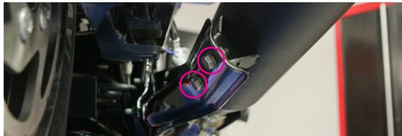
7. Tighten joint clamp and heat shield clamp.
