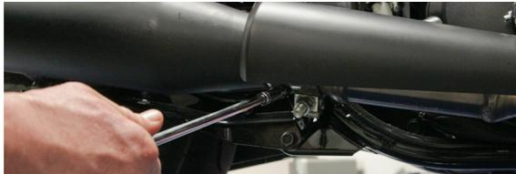
3. Remove two rear mount bolts. These will not be used with the TBR mufflers.
