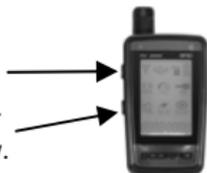
If the system was triggered, the last triggered sensor will be displayed
