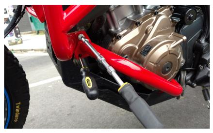
TIP! Use a screw driver or drift pin to help align all of the mount holes. This makes inserting the screws easier and helps prevent cross threading.
