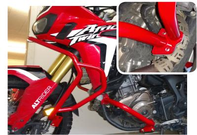
4 Slide the right and left side bars together at the center. Set them on top of the upper bracket and align the lower flanges. If you have AltRider Lower Crash Bars installed, place the upper flanges between the bracket set and lower bar flanges as shown.
