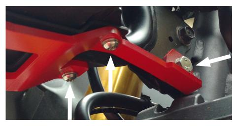
Tighten the M6 button head screws at the center bracket. (4mm Allen and 10mm wrench) TIP! Once just snug, hold the button head screw stationary, and use a wrench to rotate and tighten the M6 lock nut. This will help preserve the tool interface in the button head. Make sure bars are positioned well. Tighten the M8 hex cap screw to 18Nm
