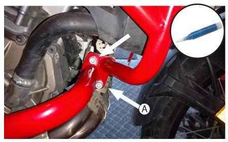
Add a drop of loctite to each M8 cap head screw. Insert M8 x 25mm long cap head screws to attach lower bars to the bracket set. In position (A) use the 18mm long screw with washers if you are mounting the upper bars only. If you have uppers and lowers use the 25mm long screw with 3 washers.
