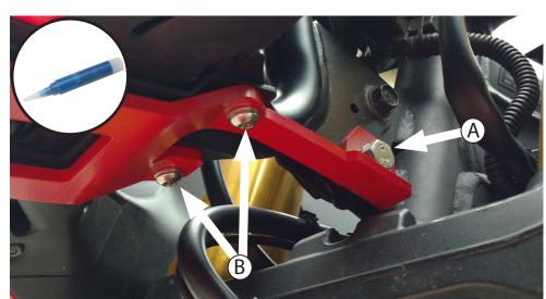
Install the center upper bracket as shown. (A) Add a drop of loctite to the M8x30 hex cap screw with washer and use 13mm socket to screw loosely in place. (B) Insert the (qty 2) M6x 20 button head screws from below (with washers) and thread on M6 lock nuts and washers on top. Leave loose for now. (If you have the headlight guard installed, leave that bracket sandwiched on top of the new crash bar bracket).
