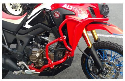
Finish Lower crash bar installation, reinforcement bar installation, skid plate installation, or headlight guard installation. Once all installations are complete, go back and make sure all fasteners have been correctly tightened.
