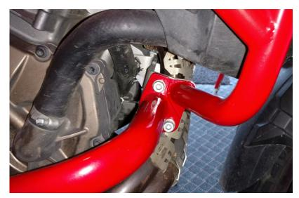
Go to step 7 in the Bracket set instructions, complete tightening of the M8 and M10 frame bolts. Then tighten the M8 socket cap screws to 23Nm
