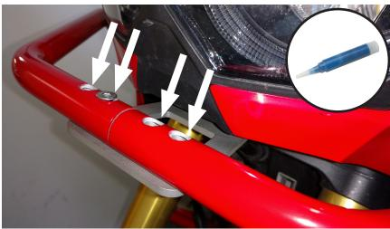
Add a drop of loctite to each M6 x 30 flat head screw and attach the bars to the upper bracket at the crossover. Tighten gradually, alternating between screws, until all are tight to 7Nm
