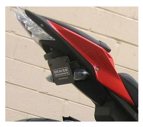
Note orientation of bracket: widely spaced holes align with undertail, license plate surface is offset and mounting holes for plate sit above where the bracket attaches to undertail
