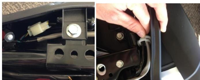
3. Remove the four nuts holding the stock fender in place and remove the stock fender. Guide the turn signal and plate light wires through, so they do not get snagged. Flip the stock fender upside down and remove the wire harness cover (there is a body rivet holding the cover in place). Once the cover has been removed, unplug the bullet connectors from the stock turn signal and plate light wires from the OEM harness. This will be reused while wiring up the turn signals.
