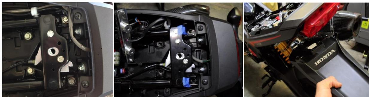
4. Remove the stock tail light by removing the two lock nuts holding it into place.
