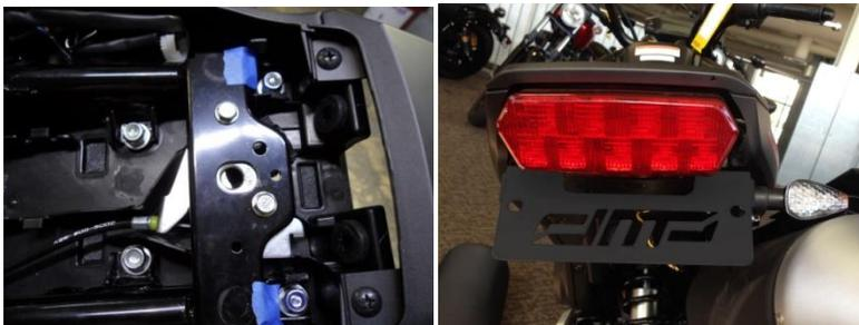
7. Mount supplied DMP market lights (900-0070). Be careful not to over tighten the market light nuts. Route the OEM turn signal wire harness and plug it in (step 2 in reverse). Plug in the DMP turn signal wires to the previously identified left and right wires from step 2. The Yellow marker light wire is the Positive lead and Negative is Black.
