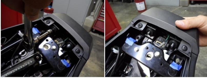
5. Install the supplied DMP base plate. Make sure the front of the base plate slides into the two slots on the undertail as well as clearing the center piece. Bolt the base plate to the bike using two of the 8x20 bolts with four of the 8mm washers and two of the 8mm lock nuts toward the front of the base plate.
