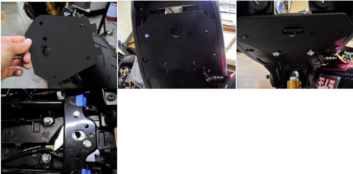
6. Install the DMP license plate bracket using two of the 8x20 bolts with four of the 8mm washers and two of the 8mm lock nuts and remount the brake light.
