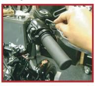
3. Loosen up the throttle and idle cables using two 3/8" wrenches. Make sure to split the upper and lower switch housing enough to clear the groove on the throttle grip then slide off the throttle grip.
