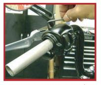
Slide on the new RSD clutch grip until the grip stops against the switch housing. Using a I/8" transfer punch and hammer, mark the set screw locations through the threaded holes in the grip.
