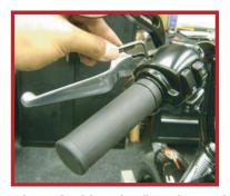
2. Use a long flat blade screw driver to break loose the adhesive between the grip and the handle bar, or cut the grip off carefully. Install the upper and lower switch housing back onto the handle bar and tighten the T25 torx screws to factory specs.
