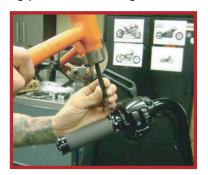
4. Remove the grip and using a I/8" center drill, drill two small dimples into the bar. These dimples will insure the grip will not rotate after the set screws are installed.
