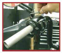
3. Slide on the new RSD clutch grip until the grip stops against the switch housing. Using a I/8" transfer punch and hammer, mark the set screw locations through the threaded holes in the grip. NOTE: On the RSD Tracker grips make sure the RSD logo is horizontal.
