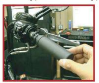
4. Slide the RSD throttle grip onto the handle bar and insert the throttle and idle able ends. Position the upper and lower switch housing on the handle bar. Tighten the 2 Torx T25 screws to factory torque specs. MAKE SURE THE THROTTLE OPERATES SMOOTHLY LOCK TO LOCK. If operation is not smooth loosen the master cylinder and throttle housing and reposition to allow for smooth function.
