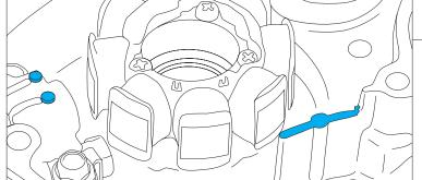
bolts! Replace the shifter. Make sure the bolt threads in smoothly - cross threading is easy.
