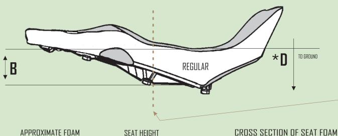
APPROXIMATE FOAM THICKNESS IN SEATING AREA: A. 2.56" (SEAT THICKNESS) B. 2.25" (SEAT THICKNESS)
