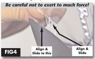
**Fig 4.** To finish the installation process, align and slide the U-hooks located upper fairing corners, into their respective slot by applying light pressure.
