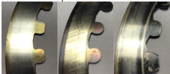
Normal Heat High Heat (Blue) Excessive Heat (Black)
